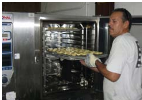
Heavily used bars are rebatched, a process wherein the soap is melted down and cooked to a temperature that completely kills any bacteria or virus. Slightly or moderately used bars are sterilized with a combination of steam and pressure.
